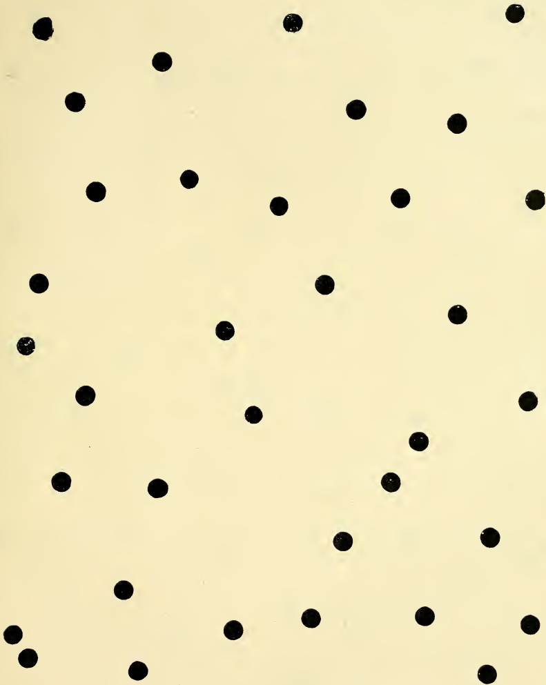
Pattern of 12-bore Choke, with 1\frac{1}{2} oz. No. 6 Shot, at 40 yards.
